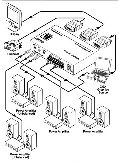
Figure 5: Connecting the VP-200NAK 1:2 XGA / Audio DA
